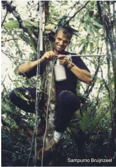
Raimond Hafkenschied installing a humidity sensor in Jamaica.
