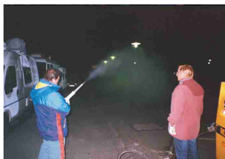
Jürgen Hofmeister with the dry ice, fog dispersal gun during a fog event. Wolfgang Wieprecht is on the right.
