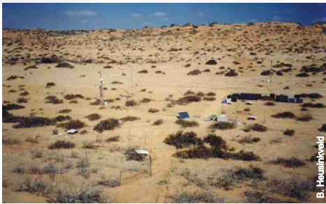
Part of the meteorological setup for dew measurements along a linear sand dune slope, Nizzana, Israel (34° 23' E; 30° 56' N; 190 m elevation).
