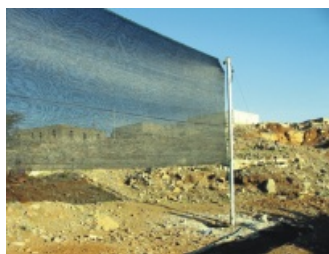
A large fog collector at Mabijan, Yemen. The trough had not yet been installed at the time of the photo.
