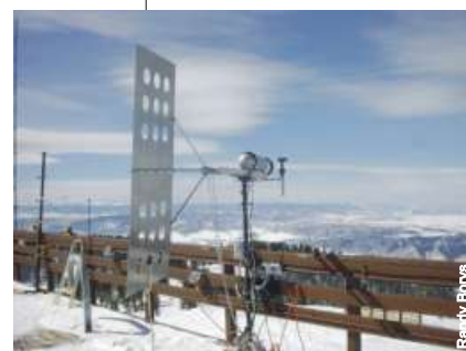
The Forward Scattering Spectrometer Probe used to measure droplet sizes and concentrations.
