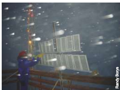
A special set of collectors for fog/cloud water used to assess the presence of bacteria in the air.
