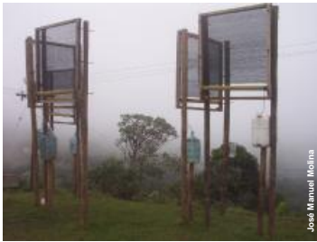
Standard fog collectors at the KM 18 site near Cali, Colombia.
