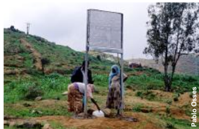
This SFC at Embatkala, Eritrea, is producing an average of 3.6 L of water a day and this is being used by the people while the measurements are being taken.
