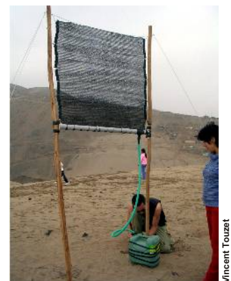
A simple fog collector constructed by a French architect, Vincent Touzet, to help an impoverished community near Lima, Peru.
