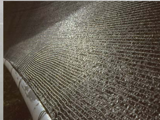
Each large fog collector produces about 200 liters of clean water a day.
