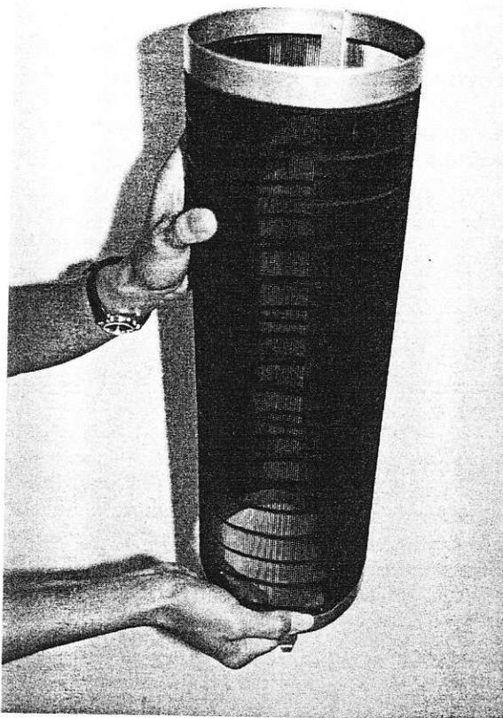
FIG. 1. An alternative fog/cloud water collector. Louvered screen collection material is manufactured from sheet aluminum (0.216-mm thickness). There are seven louvers per centimeter, each 23.1 mm long by 1.4 cm wide, angled at  $17^\circ$ . The cylinder, with louvers aligned vertically, is 12.7 mm in diameter and 40.6 cm in height ( $515.6\text{-cm}^2$  silhouette area). It is designed to mount inside the orifice of a 15-cm-diameter recording rain gauge or funnel.
