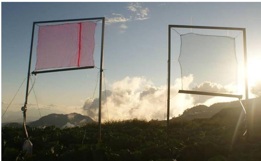
**Figure 6.** Side by Side Comparison of Fog Collectors. Raschel mesh (left) and Polypropylene mesh (right).
